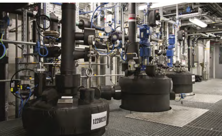
Container for precipitation of lignin from cooking liquor
