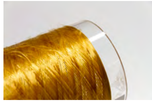
IONCELL fiber made from cellulose and Organosolv lignin
