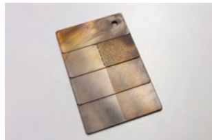
Arboblend test specimen with Organosolv lignin (Tecnar)
